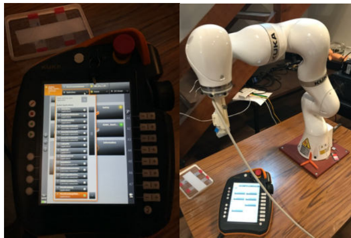
Figure 14. Left: controller of the robotic arm showing the different programs you can select. Right: robotic arm with its controller.
