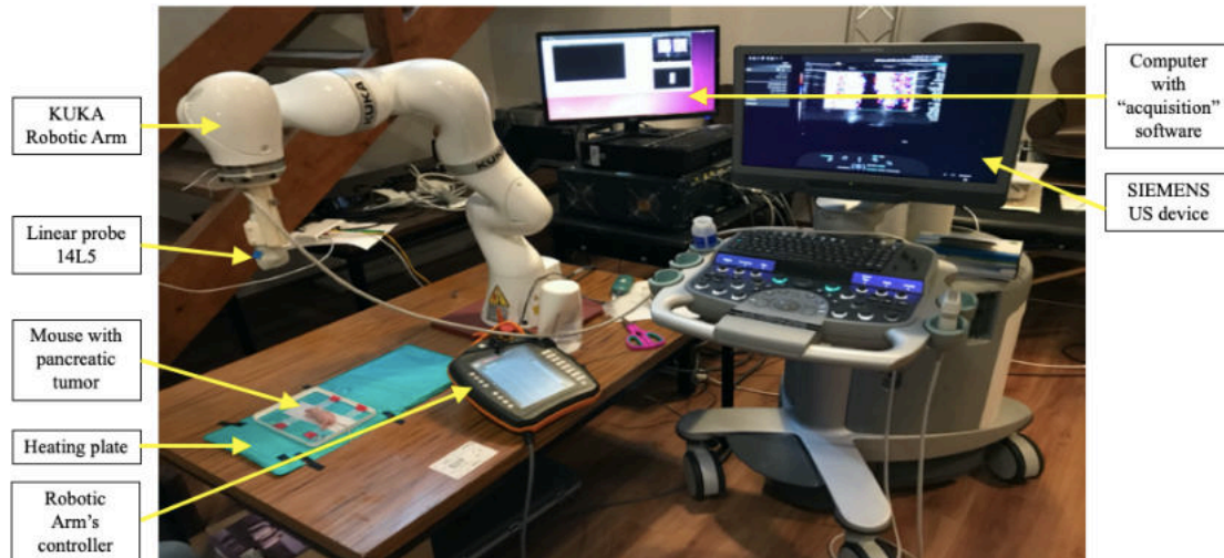
Figure 21. All the components of the product set up for a scan. Notice that both, robotic arm and US device, are connected to the computer for the scan recording.
