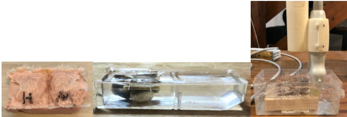
Figure 11. Left: phantom made of pigmented silicone (in the left side, a hazelnut mimicked the brain, and in the right side, water did it). Center: phantom made of transparent silicone (a grape mimicked the brain). These first two phantoms did not work because the silicone reflected all the US waves. Right: final phantom made of a bone screwed on a piece of wood and a grape mimicked the brain.
